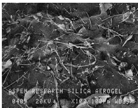
Fig. 1 SEM of silica fibers in silica aerogel.
